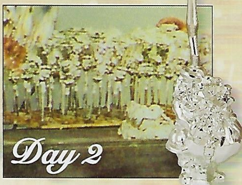
Day 2 On the second day of production, the ornament is injected with liquid sterling, another process done by hand. The silvering gives the ornaments their luminescence and sets them apart from all other glass ornaments.
